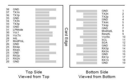
Figure 2. MSA Compliant Connector
