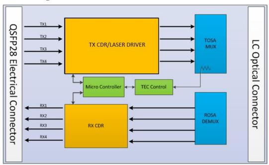
Figure 1. Transceiver Block Diagram
