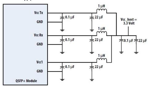
Figure 3. Recommended Power Supply Filter
