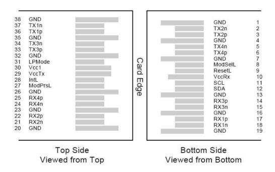
Figure 2. MSA Compliant Connector
