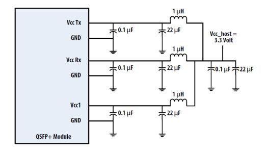
Figure 3. Recommended Power Supply Filter
